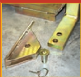
Both clamping feet are adjustable to reach longer pavers.
