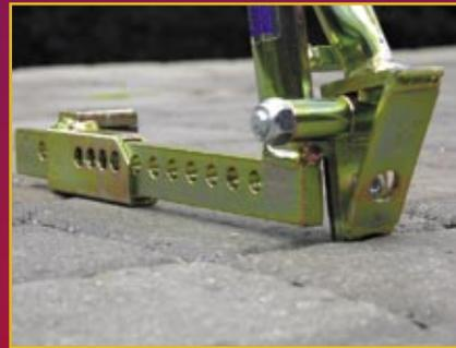
Make sure that the teeth are all the way down in the joint. The **PAVEREXTRACTOR** will touch the top of the pavers on both ends (as shown).
