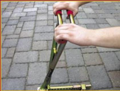
If the handles are set to close together, they will hit the stop-bar when squeezed. In this case full force can not be applied to the paver, pull out the **QUICKPIN** and reset the handles.
