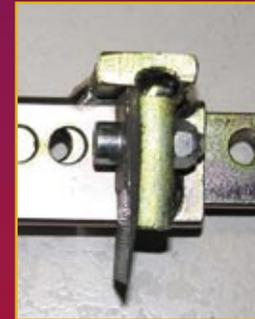
Note the slight curvature of a new tooth. If the teeth are not all the way down in the joint or the **PAVEREXTRACTOR** slips off the paver too many times, the teeth will straighten or break. In either case, the teeth will need replacement.
